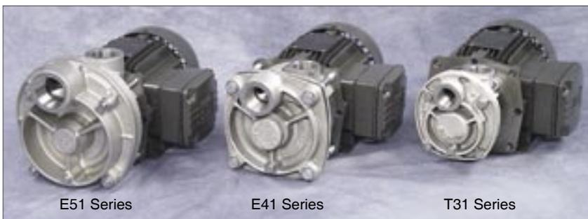
The T31, E41, and E51 Series close-coupled regenerative turbine pumps utilize our custom manufactured dual face 3450RPM D3 motors that incorporate a 304 stainless steel shaft and heavy-duty bearing. The stainless steel shaft eliminates the necessity
